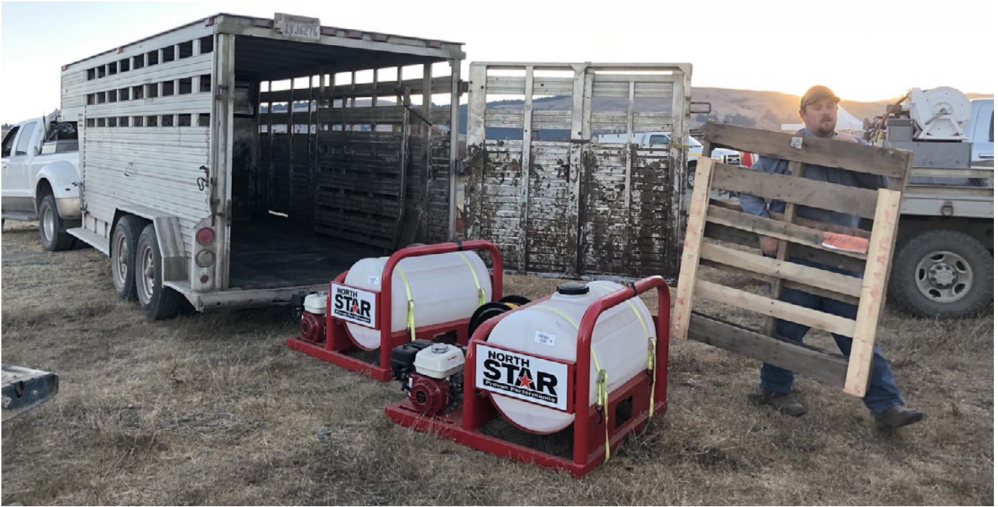
The Humboldt County PBA has two 55-gallon slip-in units that can be easily lifted by two people and used in the bed of a pick-up. In this case, a PBA member brought both units to a burn in his livestock trailer.
